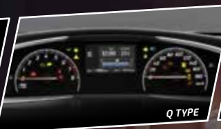
OPTITRON COMBINATION METER WITH 4.2" TFT SCREEN MID (Q TYPE)
